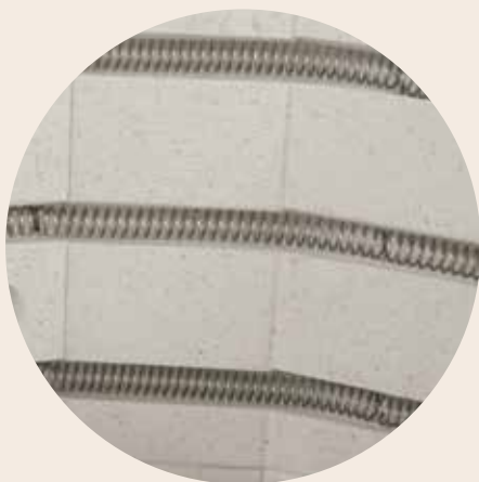
All-round heating elements, protected in grooves
