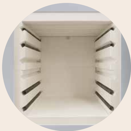
Two-sided heating with elements protected in grooves
